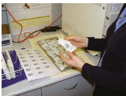
Figure 3. The tracking labels are attached to each individual bag from the autoclave (optionally, the labels can also be placed prior to autoclaving).
