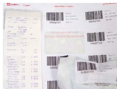
Figure 4. The duplicate label remains on the sheet and the printout from the autoclave is attached to this to correlate the steri cycle with the tracking barcodes.
